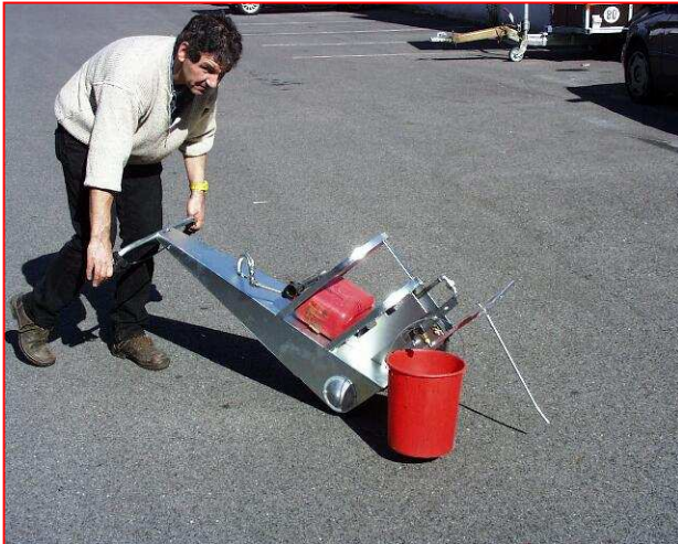
Figure 8: To clean the system: Pull spray cart backwards with the grip being pulled to pump back the primer into the can. [New Equipment: pull back the spray cart with all wheels touching the surface]
