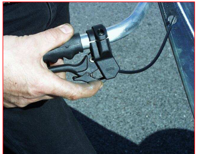
Figure 7: Grip can be fixed for spraying continuous lines [Not applicable for New Equipment]
