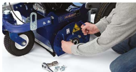
2. Remove bolts and door
