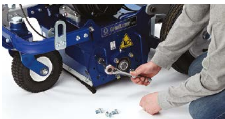
1. Loosen four bolts
